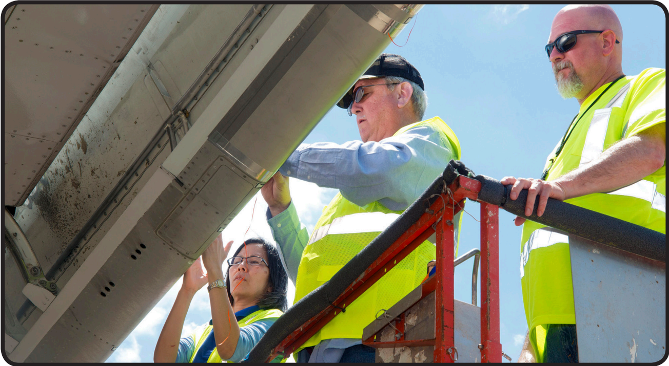
Image Caption: Materials scientist Mia Sioch (left) and systems engineer Mike Alexander (center), both from NASA's Langley Research Center, join Boeing technician Felix Boyett on a scissor lift so they can count insect residue on the right wing of Boeing's ecoDemonstrator 757 aircraft as part of NASA non-stick bug coating research in Shreveport, Louisiana. (Credit: NASA/Paul Bagby)
