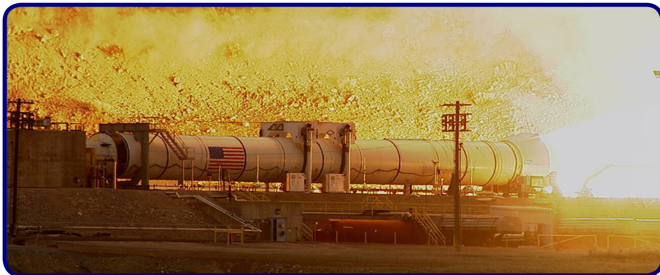
Image Caption: The first test fire of the booster for NASA's SLS rocket. (Credit: NASA)
